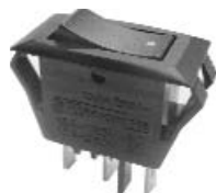
Snap-in mounting with neon indicator. 15A @ 125VAC. Mtg. hole: 29 x 13mm
