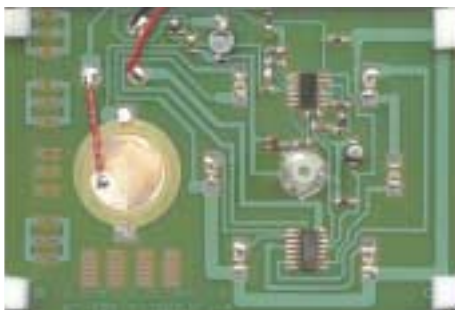
SM-200K PCB board showing practice areas & mounted components
